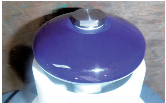
Glass Disc with Temperature Sensor underneath a tantalum cap
