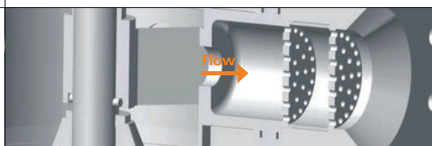
Nozzle plates in bypass letdown unit
