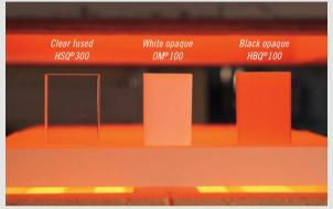
${\it HBQ}{}^{\it s}100$  exhibits high — silicon like — emissivity combined with low thermal conductivity
