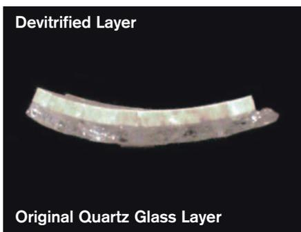
High cristobalite has nearly the same density as glassy silica and thus cannot be seen on the surface. However, upon cooling, high cristobalite undergoes a structural change from a cubic to a tetragonal crystal structure at about 275°C. This is accompanied by a large decrease in density that can result in some cracking and spalling. Refractive index differences resulting from the birefringent tetragonal crystal structure also cause the devitrified spots to turn white.
