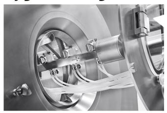
The new spray boom design was developed with the spray nozzle specialist Schlick and is basing on the established PCA System. In order to limit the tubing in the internal machine within reasonable limits and to increase cleaning ability, supply lines for spraying-, pattern- and control- air are elaborated as boreholes through the arm.
