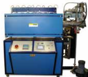
Sublimationsöfen zum Sublimieren von Material zur Materialreinigung. Sublimation furnace for sublimation of materials for the purposes of material purification.
