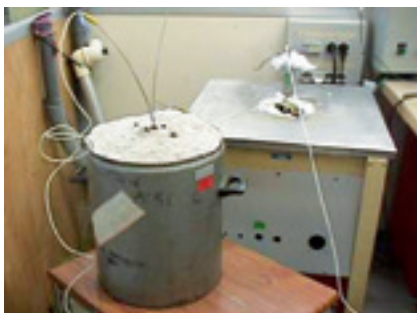
Calibration by comparison: salted bath
