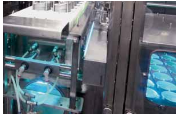
UV disinfection of pre-stamped sealing films
