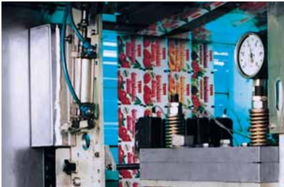
UV disinfection of sealing films
