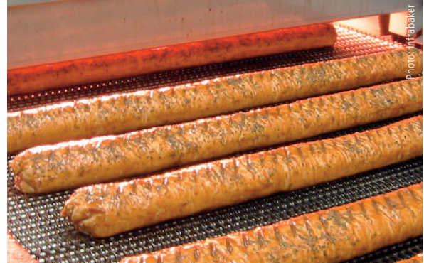
Infrared is used to brown chicken meat for sandwiches
