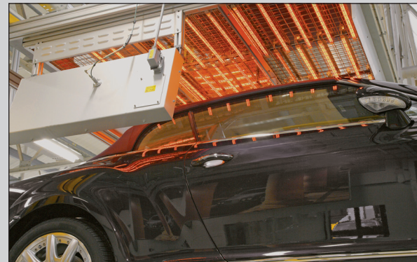
Crease removal of synthetic fabric
