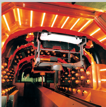
Curing paint on plastic bumpers
