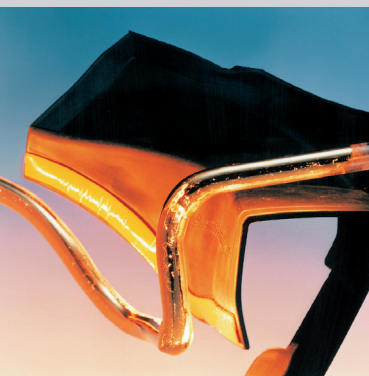
Activating adhesive on a rubber sleeve with contour infrared emitters
