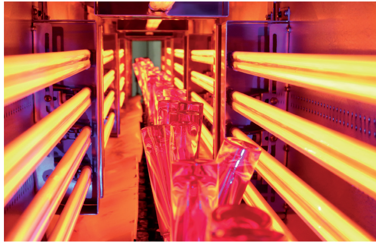
Curing of coatings on glass bottles
