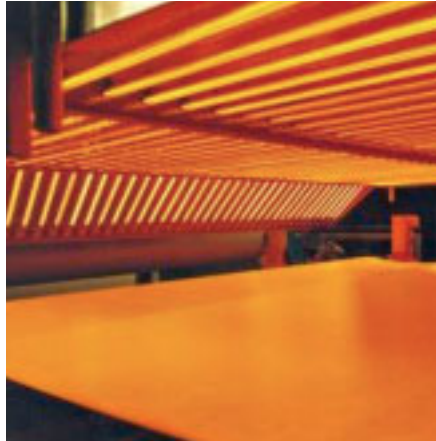
Embossing Infrared provides fast and targeted surface heating before embossing.
