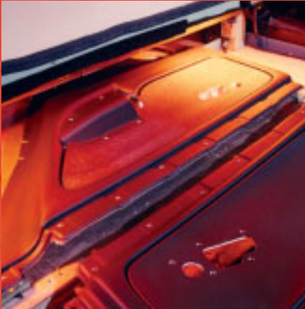
Activation of adhesives Infrared heat ensures that adhesives are activated precisely where required.
