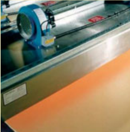
Blinds Pre-heating prior to stenter
