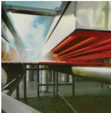
Polypropylene fibres Heating for melting/fusion
