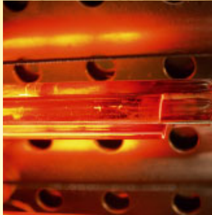
Thread and yarn Drying with a slot emitter
